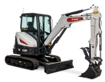
e high-performing Bobcat E35 compact (mini) excavator features 33 hp engine for more usable power.
